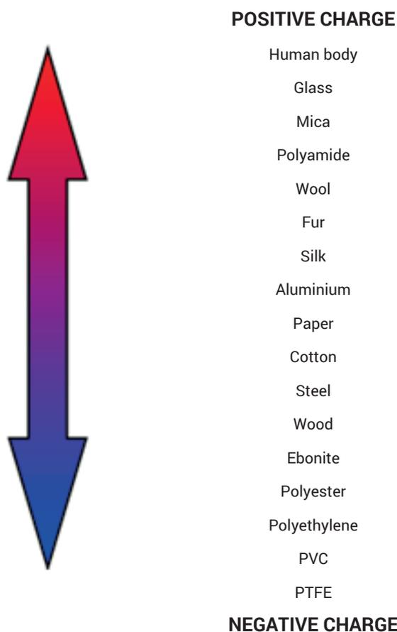
Figure 6. The triboelectric series
