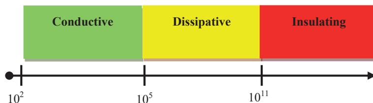
Figure 5. The division of materials in terms of electrostatic properties
