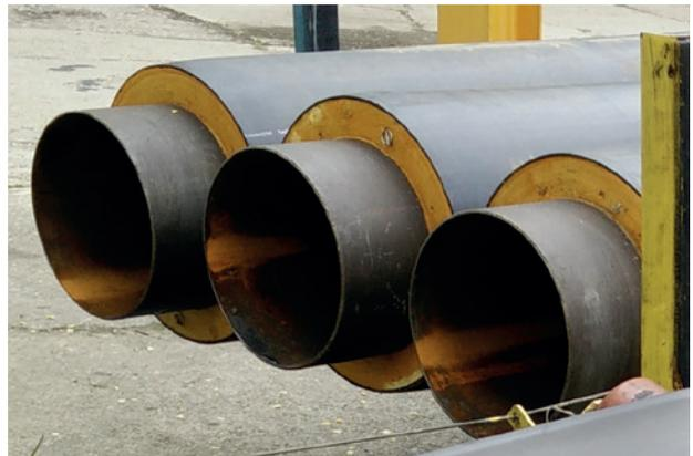
**Figure 1b.** Manufactured pre-insulated pipes
