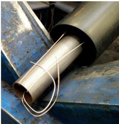
**Figure 1a.** Manufactured pre-insulated pipes
