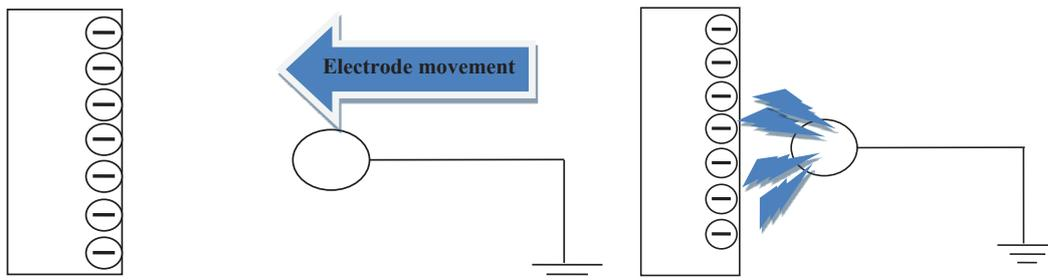
**Figure 2.** Typical brush discharge occurrence conditions (scheme)
